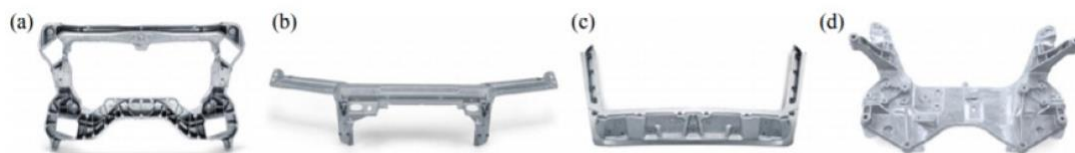
(a) Car engine bracket ; (b) The front frame of the car ; (c) Automobile tailgate frame ; (d) Automobile chassis components (8)
